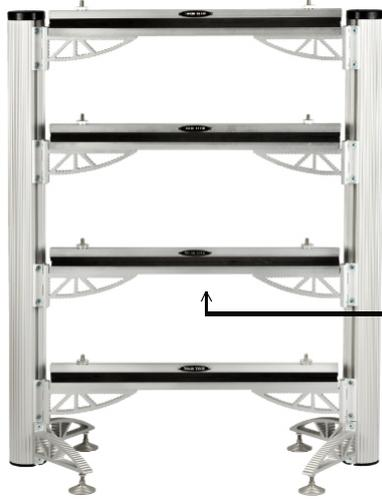
The Cable Rack can handle cables of a maximum diameter of 3,5 cm. Combining different sizes of cables in the same carrier is possible but the difference should preferably not be more than 1 cm in diameter. If the difference is larger than 1 cm it is recommended to use one carrier for the thick size and another for thin cables.
